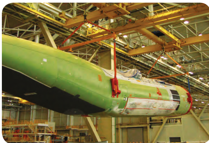
MULTIPLE POINTS UNDERSLUNG TANDEM WORKING CRANES 多吊点同步运行悬挂起重机
